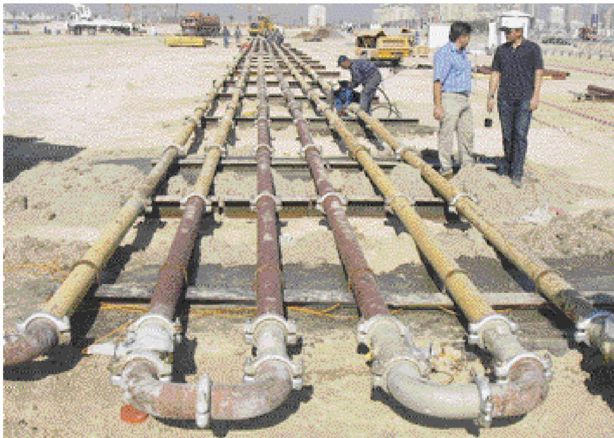
To simulate high-rise concrete delivery under extreme conditions, hundreds of metres of delivery line were first laid horizontally, measurement values and factors such as friction coefficients were determined and converted to high-rise pumping.
