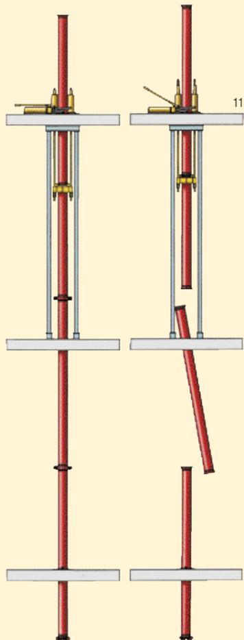
Changing the pipeline using the hydraulic lifting mechanism
